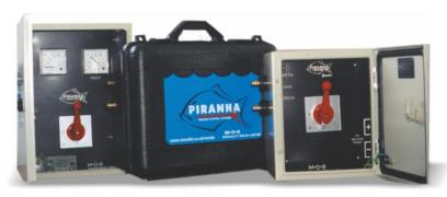
The Piranha<sup>™</sup> (I) welding control unit is a 400 amp DC isolating switch, monitoring and control station, allowing for safe isolation of the welding current and voltage. Each unit is fitted with amp and volt meters and DIN style quick release cable connectors (supplied) and a large, easy to use switching handle. Designed to sit between the machine and the operator, the device allows for monitoring and control of
