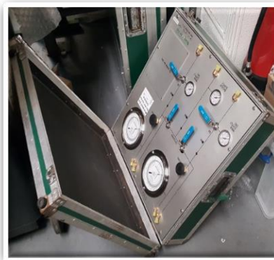
Mobile Boxed 2 Diver LP Panel with built in Comms box option (not shown)
