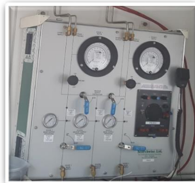
Mobile Boxed 2 Diver LP Panel with built in Comms box option (not shown)
