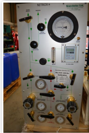
3 Diver Panel; 2 x HP Nitrox Modules (with LP Air Intervention) & 1x Standby Diver Air Module
